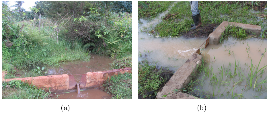
Figure B.4: V-notch weir for discharge measurement of Tegu Stream, Kenya: (a) Normal condition, upper weir; (b) Overflow of lower weir during rainy season.
