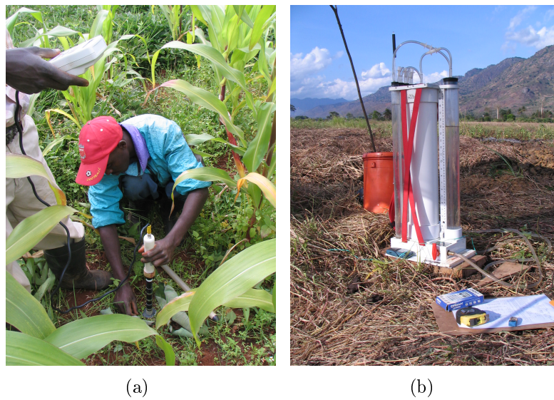
Figure B.2: Measurement devices for soil moisture and saturated hydraulic conductivity: (a) Profile Probe PR2 with handheld device HH2; (b) Compact Constant Head Permeameter.
