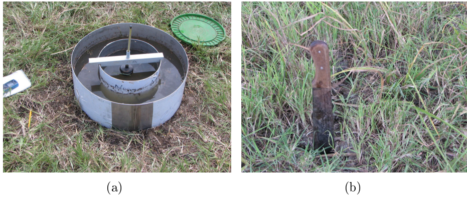
Figure B.3: Double-ring method for in-situ measurement of infiltration rate: (a) Application of double-ring method; (b) Cracks at grazing site in floodplain, Tanzania.
