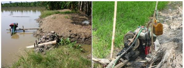
Picture 5-3. Individual diesel pump used for collective pumping; Right – pump with fuel can (Huynh Linh 2011)
