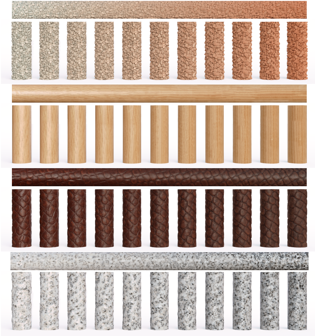
Figure 10.7: Example interpolations between measured materials. The horizontal cylinder shows a continuous interpolation sequence between the materials. The vertical cylinders each feature a synthesis result at one discrete interpolation step. The images are generated using monte-carlo path tracing with an environment-illumination and an additional point-light source to emphasize highlights. Further results are shown in Figure 10.8.
