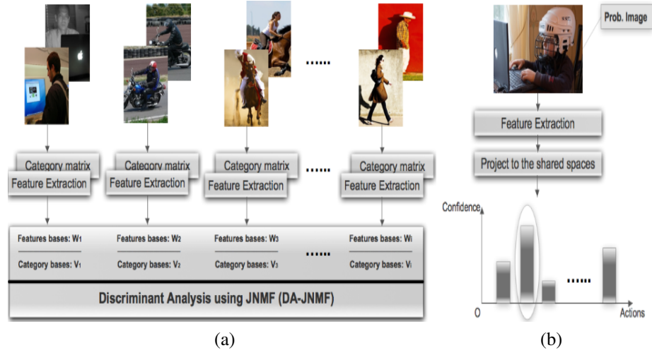
Figure 3.1: General diagram of DA-JNMF classification for (a) training on ground truth data and (b) testing on new samples
