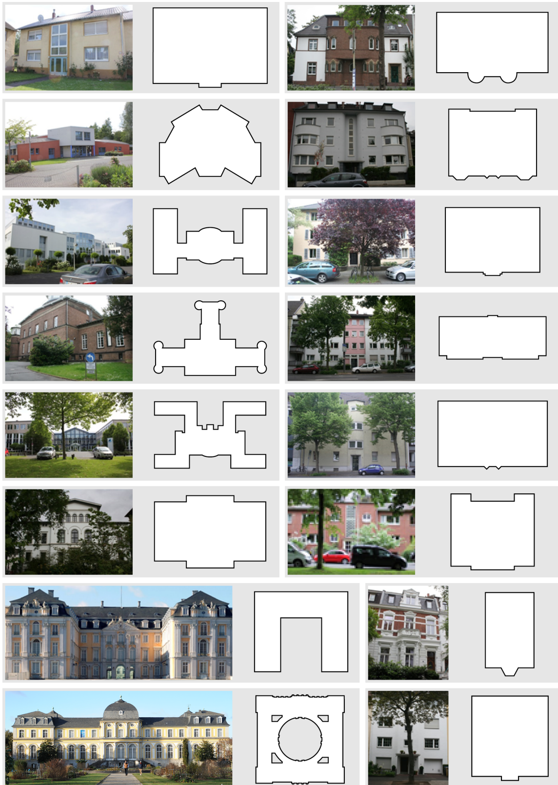
Figure 3.9: Examples of façades and their corresponding footprints. The symmetries of the façade can already be derived from the footprint symmetries.
