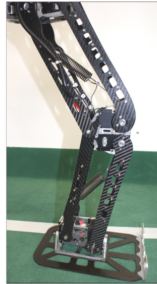
Figure 3.3: Parallel kinematic leg design.
