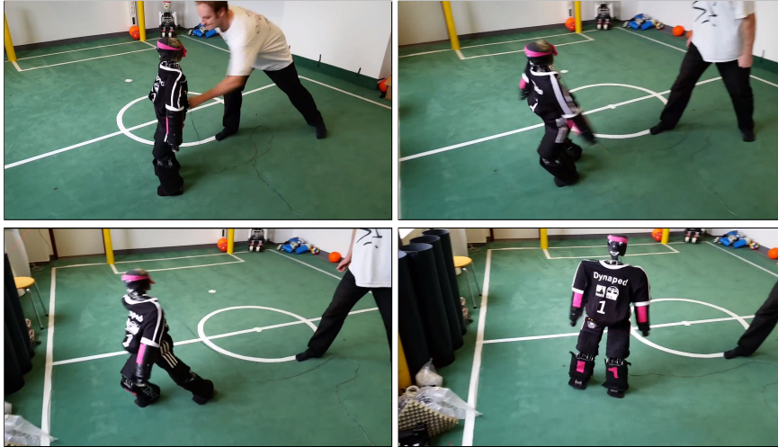
Figure 8.9: Extreme push recovery with bipedal robot Dynaped.
