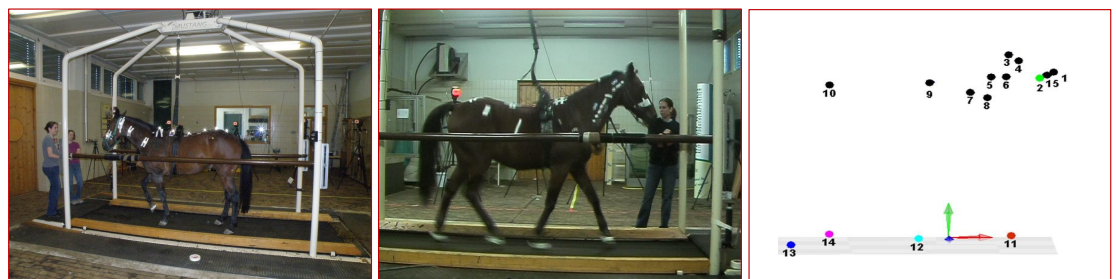
(a) MoCap environment (b) Marker setup (c) 3D markers' visualization
