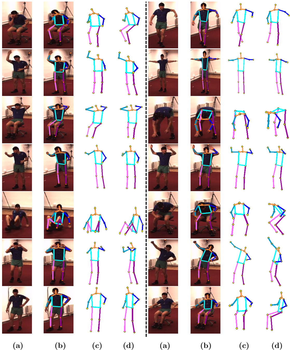
Figure 7.9: A few qualitative results from Human3.6M dataset [IPOS14]: (a) represents input images, (b) shows refined 2D poses while (c) and (d) correspond to estimated 3D poses from two different views.
