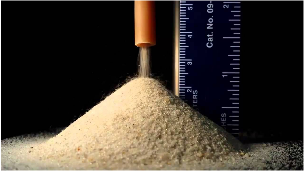
Fig. 7.3: Sand rilling from an outlet. A typical conical pile evolves and forms the critical angle of repose, which could be extracted from this experiment.
