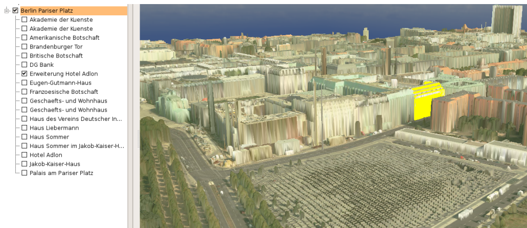
Figure 6.2: Screenshot from the rendering application showing a highlighted feature of the semantic dataset within a visualization of the Berlin DSM.
