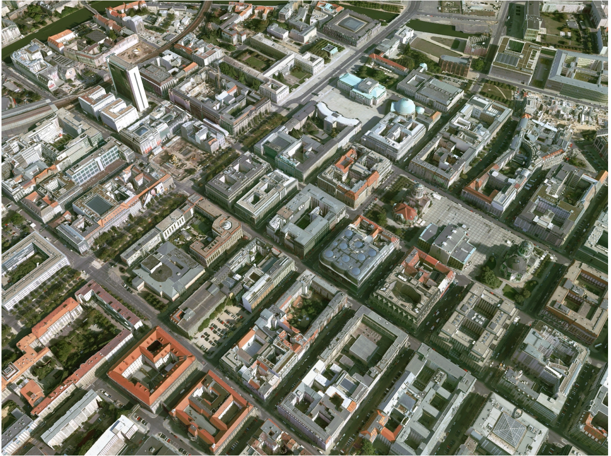
Figure 5.1: Rendering of the automatically reconstructed city model of downtown Berlin on top of a corresponding DTM.
