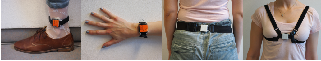
Figure 7.1: Placement of four APDM Opal IMUs on different body parts. The sensors were placed on four different locations: left ankle, right wrist, lower back, and chest.
