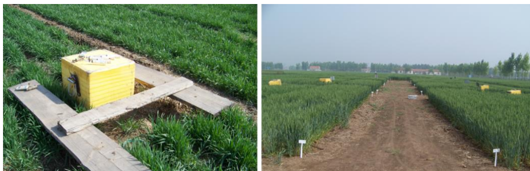
Figure 2. Static chamber used in field experiments described in Paper IV and VIII.
