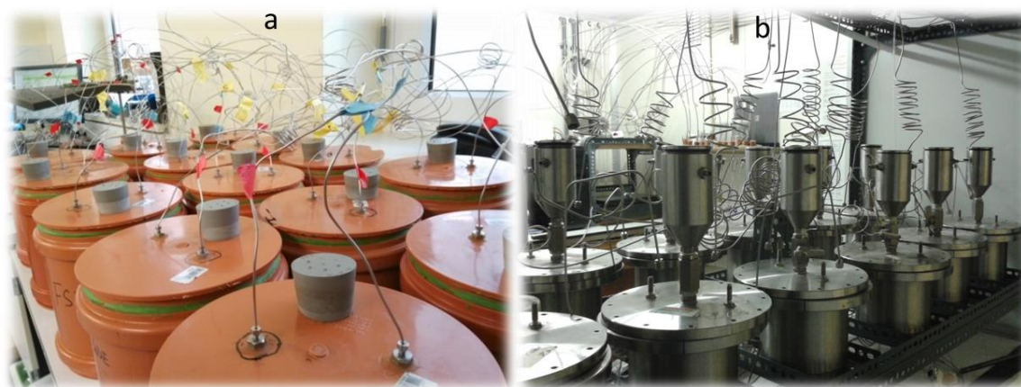
Figure 3. The two automatic incubation systems (a) used in Paper II and V and (b) used in Paper I and III.
