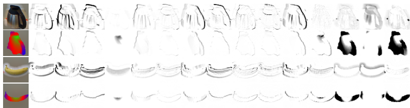
Figure 8.5: CNN activations for sample RGB-D frames. The first column shows the CNN input image (color and depth of a pitcher and a banana), all other columns show corresponding selected responses from the first convolutional layer. Note that each column is the result of the same filter applied to color and pre-processed depth.
