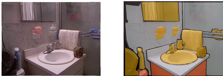
Figure 6.1: Object class segmentation example from the NYUD. Left: input image. Right: input overlaid with ground truth pixel-wise labels (walls, furniture, objects). Black regions in the ground truth are unlabeled and do not contribute to the loss.
