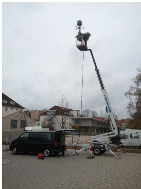
Figure 6.36: Picture of the OS © 2013 Saab Medav Technologies GmbH. The antenna array is carried by a lifting platform with a height of 10m.
