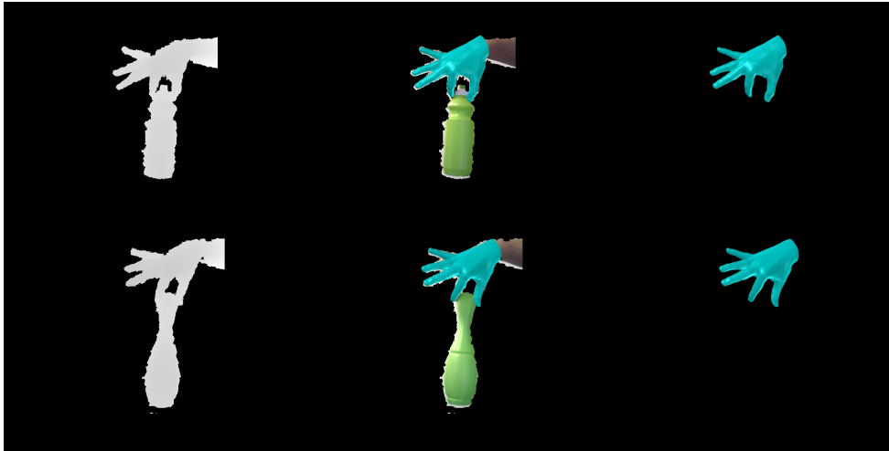
Figure 5.2: The hand tracker used in the in-hand scanning pipeline. The left image shows the raw depth input map, the middle image shows the hand pose overlaid on top of the RGB-D data, while the right image shows just the hand pose.
