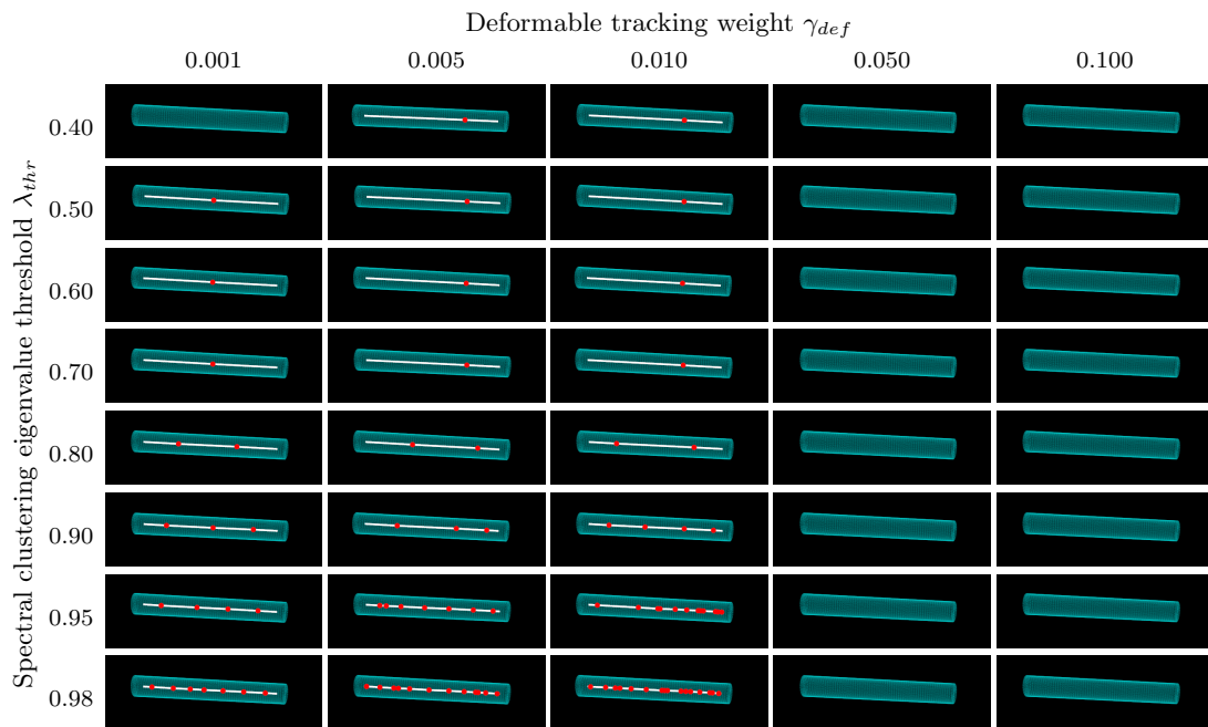
Figure 6.16: Results for all configurations (\gamma_{def}, \lambda_{thr}) that arise from the proposed parameters. The images show for the object “pipe 3/4” the inferred 3d skeleton, where the joints with DoF are depicted with red color.
