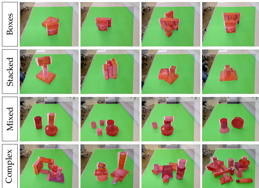
Figure 2.15: Example segmentations for OSD v0.2, the semantic object detection dataset (Richtsfield et al. , 2012). The detection results are shown as semi-transparent overlays over the original RGB images with invalid depth measurements (white), support surface (green), and object candidates (red). Despite some minor deviations at object boundaries, all pixels belonging to an object in the ground truth data are correctly detected as object candidate points.
