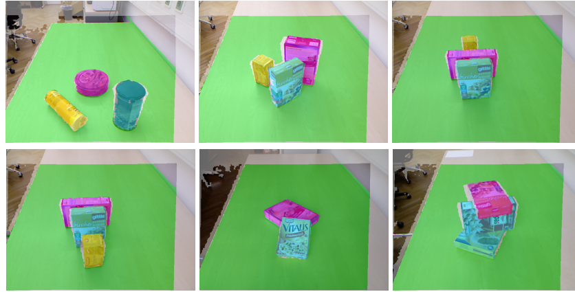
Figure 2.14: Examples of detected tables and objects in the OSD dataset by Richtsfeld et al. (2012). Shown are the original RGB input images with a color overlay encoding pixels with no depth information (white), table plane (green), and objects (randomly colored per object). Despite objects being clustered together (bottom right), all objects are reliably detected and clustered.
