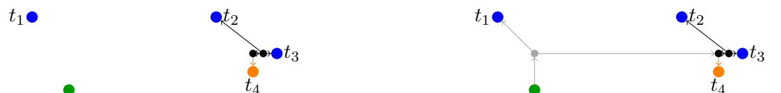
(a) Branching B after applying Optimization 5.17. The delay on the critical path to t_4 did not increase.
