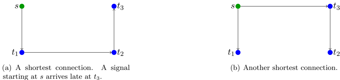
Figure 1.1: Two shortest connections of the pins consisting of horizontal and vertical wires only. Without taking timing constraints into account we might choose the left solution in which the signal starting at s arrives late at t_3 .
