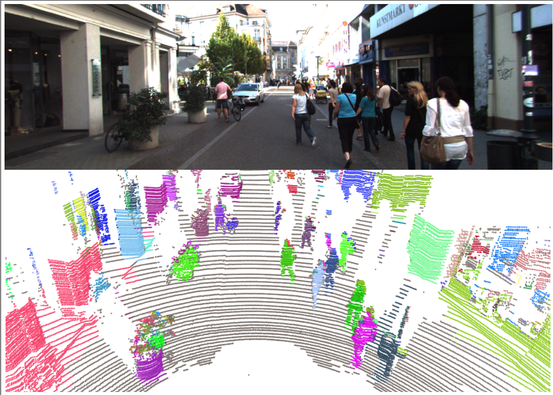
Figure 5.10: An example segmentation of a group of people from KITTI dataset. Top : an RGB image that shows the scene, shown for visualization purpose only. Bottom : the scene segmented with our algorithm. Different clusters are assigned random colors.
