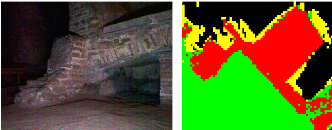
Figure 4.9: A situation in which the ground level is flat and traversable but the height of the platform prevents the robot from entering the niche. Left : RGB image from the Microsoft Kinect. Right : traversability estimate.
