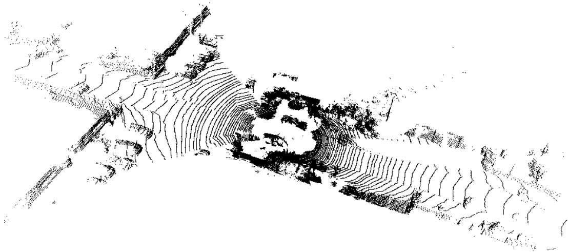
(a) laser scanner data
