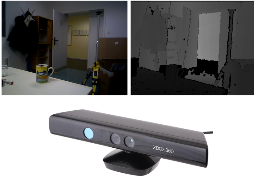
Figure 7.2: Microsoft Kinect, a RGB-D camera which can provide color (RGB) as well as depth (D) images.
