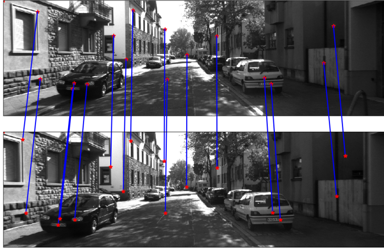
Figure 5.1: 2D-to-2D corresponding image points.
