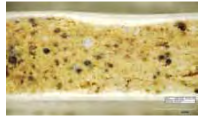
Sample ID 3549, Ware 14 rounded black particles (and transparent particles)
