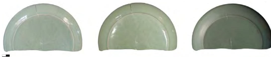
Figure 94: Problems in the depiction of colors on sample ID 2170. The first two pictures from the left are taken on the same day with the same camera and the same lamps. Only the angle of the light incidence is slightly changed in between both pictures. The picture on the right is taken with a different camera under different light conditions on another day.
