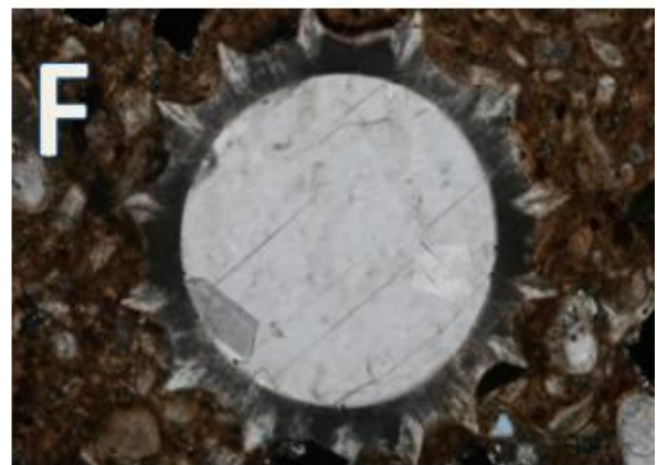
Photo micrographs showing the texture and non-plastic inclusions in sample UJ257. E: beautiful intact microfossil sun like shape by (PPL) mode, image width 0.5mm. F: same image by (CPL) mode, image width 0.5mm.
