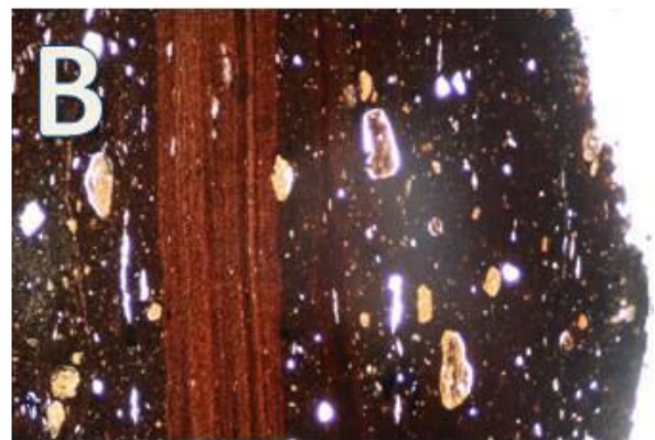
Photo micrographs showing the texture and non-plastic inclusions in sample UQ115. a: mixing two types of clayey materials by (PPL) mode, image width 4mm. b: same image but in (CPL) mode, image width 4mm.
