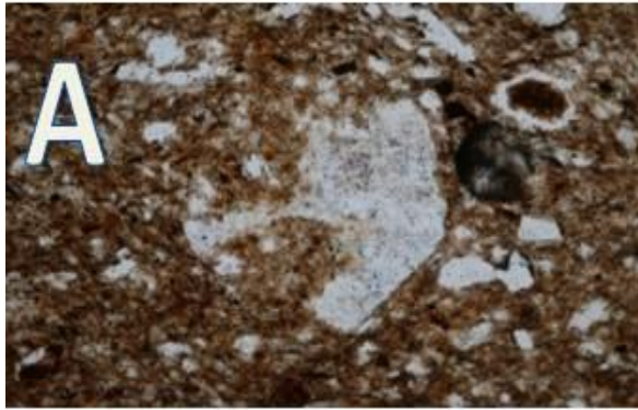
Photo micrographs showing the texture and non-plastic inclusions in sample UQ127. a: k-feldspar in a matrix contain bearing quantity of reddish iron spots by (PPL) mode, image width 0.5mm. b: same image but in (CPL) mode, , image width 0.5mm.
