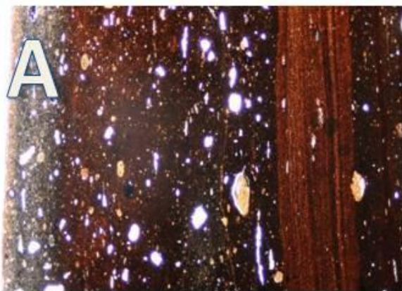
Photo micrographs showing the texture and non-plastic inclusions in sample UQ115. a: mixing two types of clayey materials by (PPL) mode, image width 4mm. b: same image but in (CPL) mode, image width 4mm.
