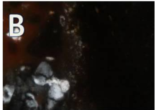
Photo micrographs showing the texture and non-plastic inclusions in sample UQ4. a: fine matrix highly sintered contains rounded inclusions clasts by (PPL) mode, image width 1mm. b: same image but in (CPL) mode, image width 1mm.
