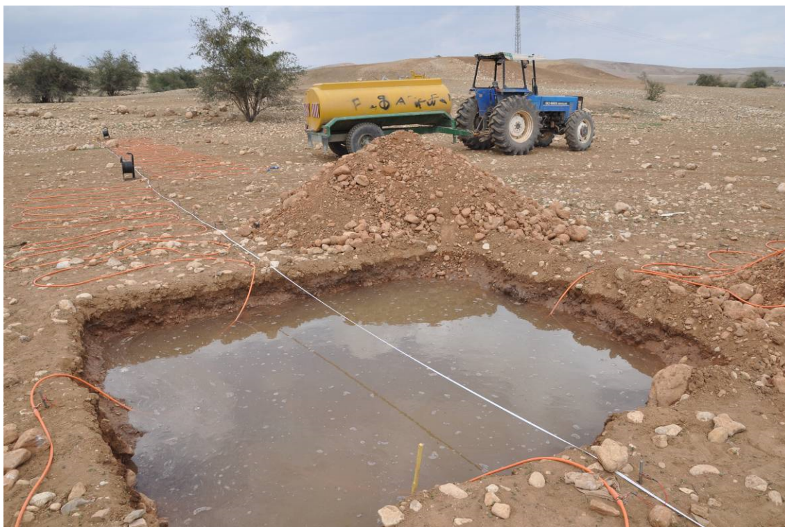
Figure 4.12: Excavated pond for the infiltration experiment, filled with water. The depth of the pond was around 0.5 m. The photograph also shows the orange cables of the IRIS Instruments Syscal measurement device for geoelectrical monitoring.
