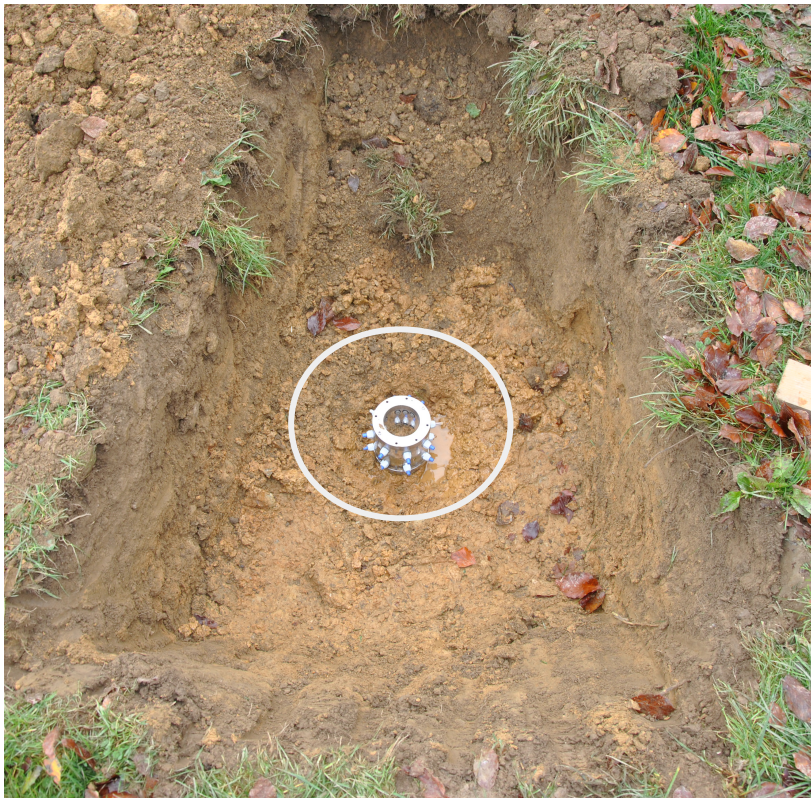
Figure 7.6: Sample collection at the Rollesbroich test site. The sample container (white circle) is pressed into the ground and later extracted together with the soil sample.
