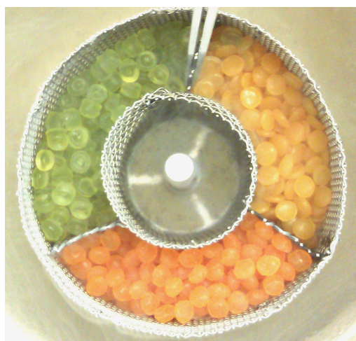
Figure 8.9: Irradiated PE and PP pellets.
