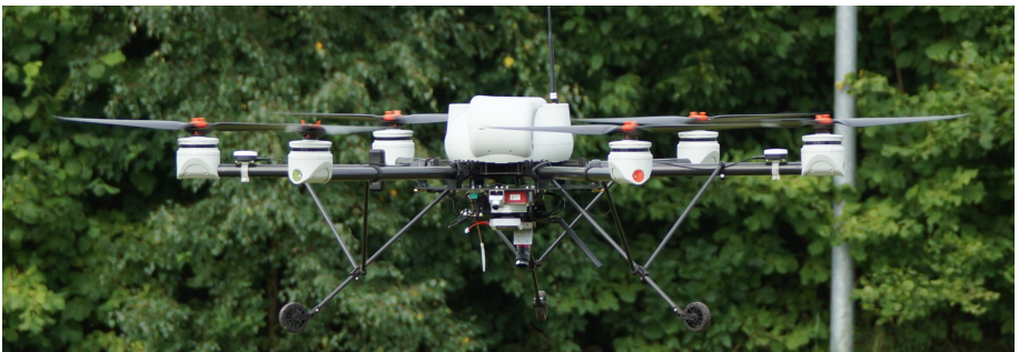
Figure 4.11: Hexacopter of the type AR-200 from AirRobot® GmbH & Co. KG equipped with the multi sensor payload.
