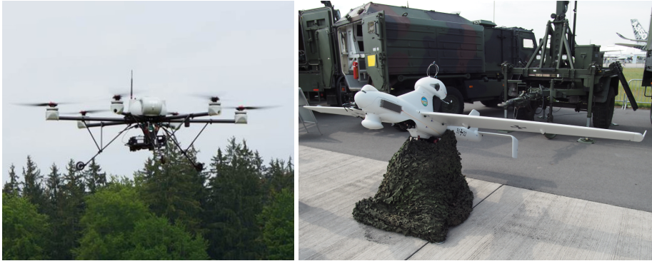
Figure 1.1: Left: Example of a rotary wing drone. The hexacopter of the type AR-200 is produced by AirRobot® GmbH & Co. KG. Right: Fixed wing drone of the type LUNA from EMT Ingenieurgesellschaft. The UAS is currently used by the German Army.
