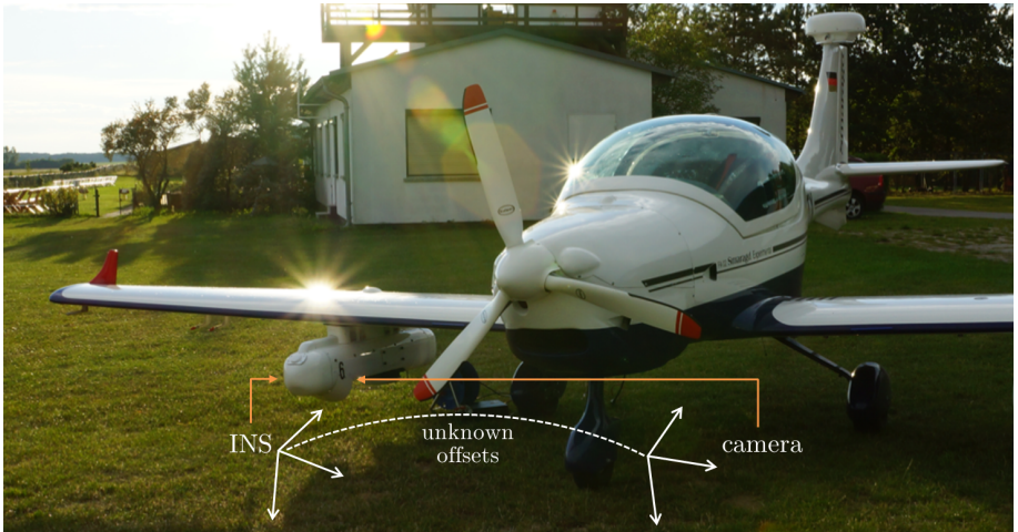
Figure 3.8: The calibration of the static coordinate system offsets between an INS and a camera enables the direct georeferencing of images collected with aerial platforms. For the flight experiments the sensors were integrated into a payload pod, which was mounted beneath one wing of a manned ultra-light airplane.
