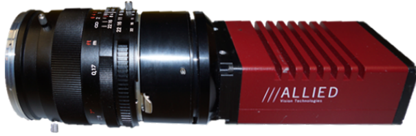
Figure 2.4: Industrial camera Prosilica GX3300 from Allied Vision Technologies GmbH with an attached wide-angle lens from Carl Zeiss AG. The camera allows grabbing the images in real-time via a standard Ethernet port while the image exposure can be externally controlled via a signal connected to a trigger jack.
