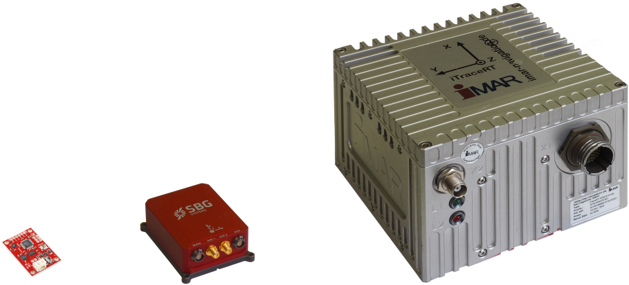
Figure 2.6: Approximated visualization of the size ratio between three selected INSs. Left: Razor IMU from SparkFun Electronics Middle: Ellipse-D from SBG Systems Right: iTraceRT-F200-E from iMAR Navigation GmbH
