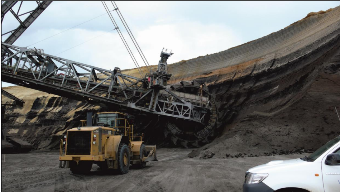
Fig. 2-2: Bucket-wheel excavator in the Garzweiler open-cast mine, removing upper parts of the Neurath Sand.
