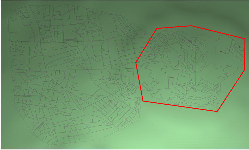
Figure 4.9: Topography Example: The example was generated using a sample from San Francisco (Mount Davidson Park, Mount Sutro) and Copenhagen. In the area enclosed by the red polygon, fragments from San Francisco were chosen because of the similar topography distribution. Notice that in this hilly area, the street pattern style differs drastically from the street pattern style in other parts in the urban layout.
