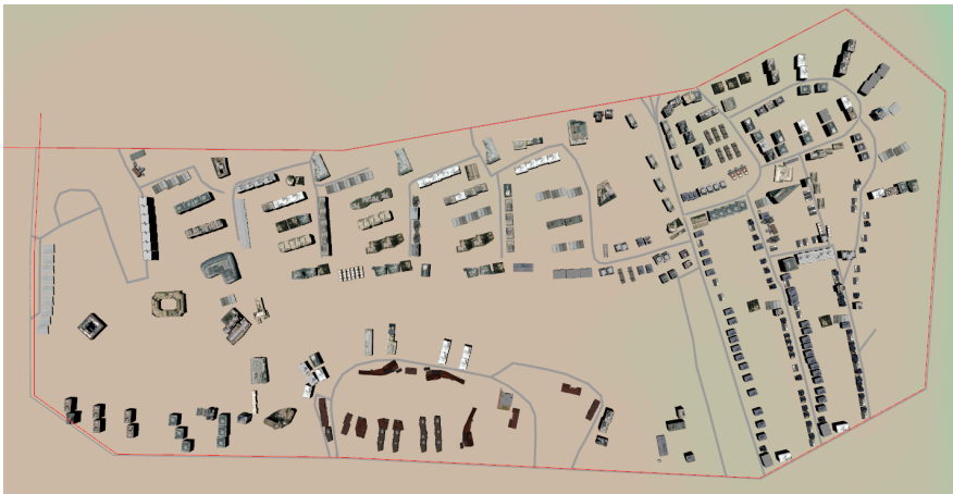
Figure 4.6: The reproduced look of a district of a real-world example city: Red sketched arterial streets serve as input. The recursive fragment synthesis algorithm faithfully reproduces the look of the region shown in Figure 4.1. Notice that even the style of building footprint layout is similar when compared to the original layout. The 3D building models were placed using the technique presented in section 5.1
