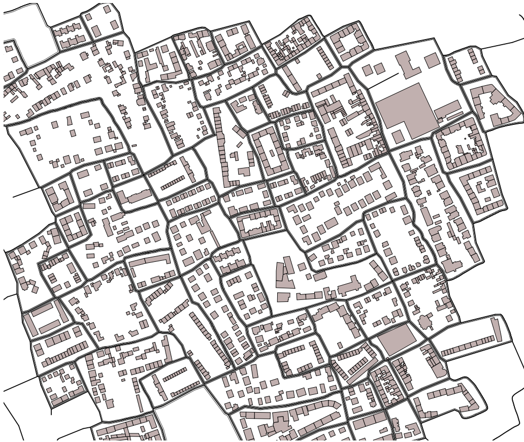
Figure 5.12: A street network that was generated by StreetGAN (section 4.2) is filled with city blocks from various German cities. Near rectangular city blocks even with wavy street segments are filled with plausible footprint layouts. Due to a small variety of irregularly shaped city blocks within the database, the synthesized city blocks are less likely in irregularly shaped blocks, because several building footprints are removed that were partially located outside the city block polygon.
