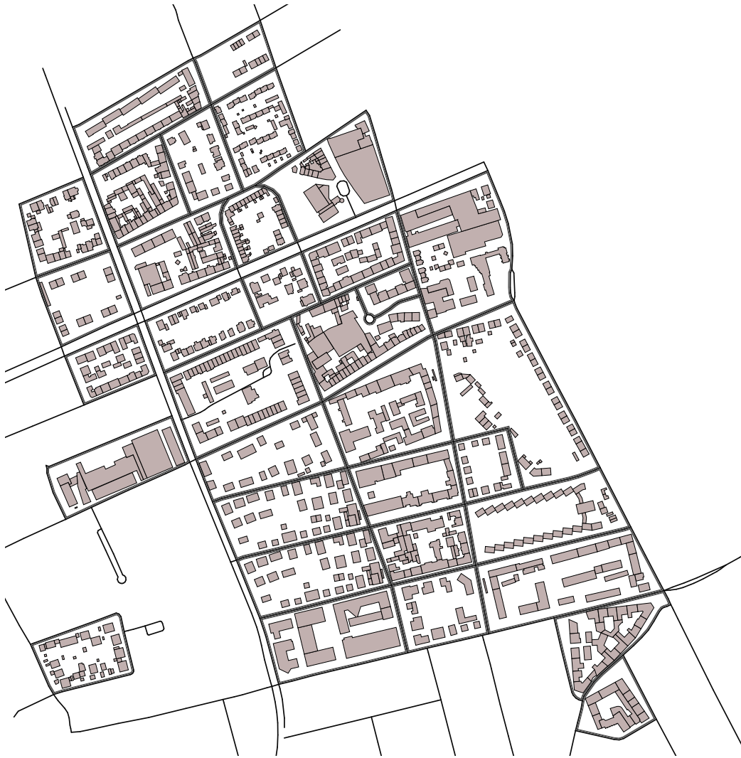
Figure 5.8: A city block layout filled by re-using exemplar city blocks from German cities: Bonn, Bremen, Frankfurt, Munich, Nürnberg. For adjacent rectangular shaped city blocks, plausible and realistic layouts are achieved using the city block layout transfer algorithm. For irregularly shaped blocks the result strongly depends on the richness of the exemplars present in the database.
