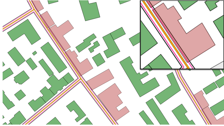
Figure 5.3: Conflicted building footprints (grey) that are partially placed on road and pavement
