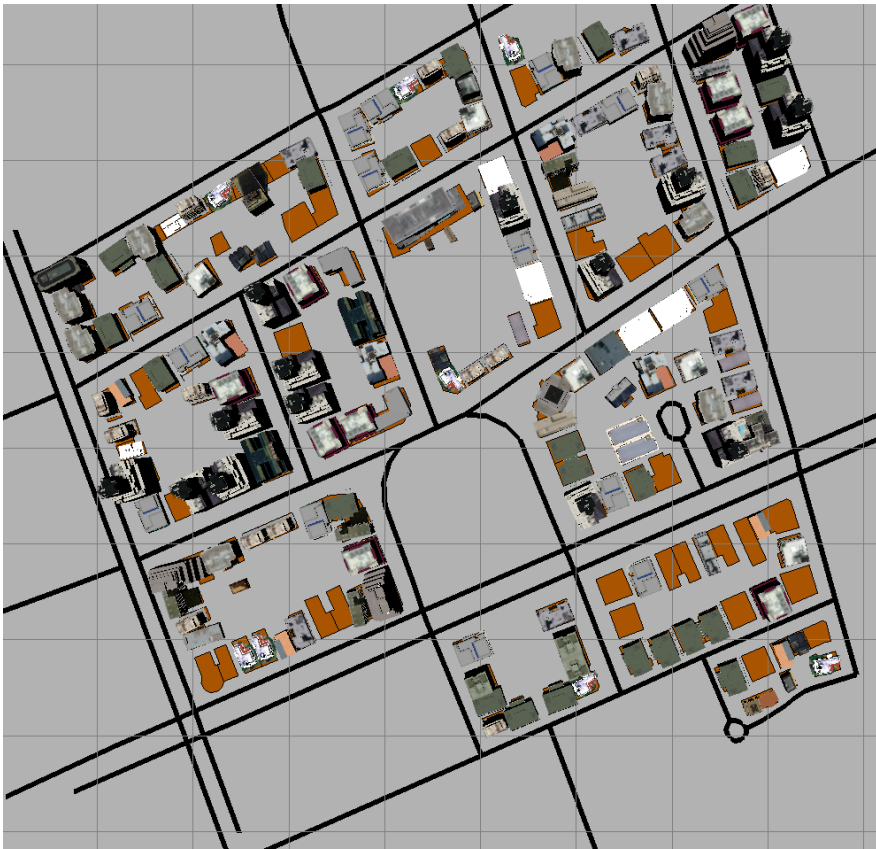
Figure 5.15: The same building footprint layout shown in Figure 5.13. In this experiment, a different similar sized database was chosen. The result of the building placement strongly depends on the shape variety present within the footprint of the 3D building models. About 14 % of place buildings to do not pass the overlap check discussed in section 5.1.5.
