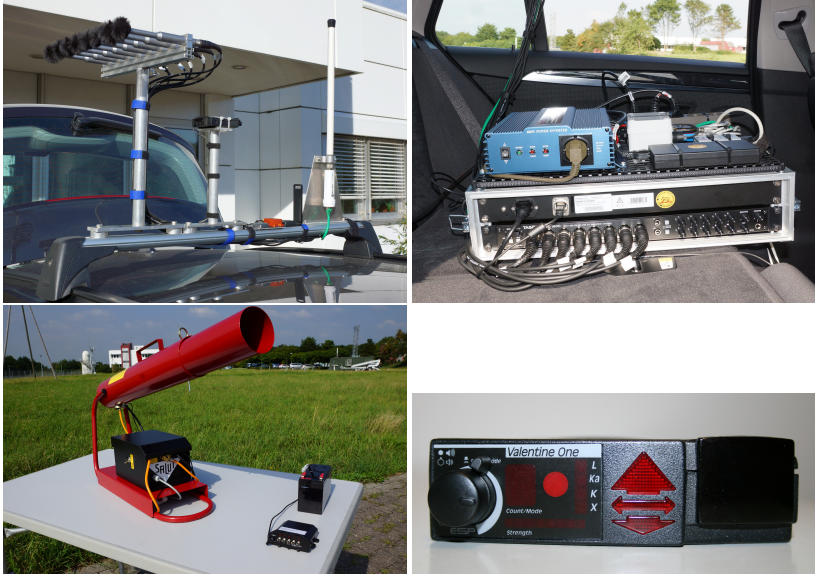
Figure 1.4: Hardware for field tests. Upper left: Microphone array, radar warner, XSens, and bullet mounted on car. Upper right: Power supplies and sound card mounted inside car. Lower left: Sonic blast-shock cannon and radar warner trigger. Lower right: commercial off-the-shelf radar and laser detector “Valentine One”, © 2016 IEEE.
