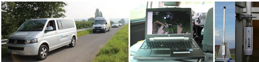
Figure 6.11: Formation of four cars during communications field tests with mounted communication devices (left), laptop with visualization and fusion software (center), and Ubiquiti Bullet M5 Wi-Fi radio device (right), © 2016 IEEE.
