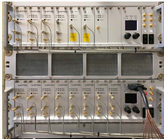
Figure 3.26: GREAT FFT Spectrometer, with 27 independent backend channels. In the image, the 12 dual input dFFTS4Gs and three single input FFTS4G boards are visible. Card ID is assigned from left to right, starting from the bottom sub-crate.
