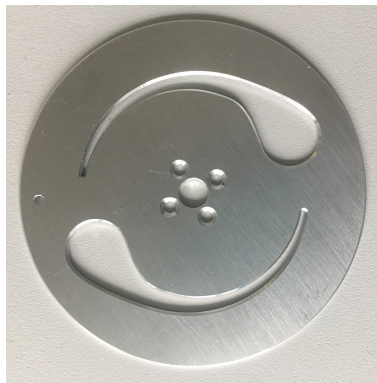
Figure 3.20: 4G-1 LO Attenuator: rotary variable pupil, a.k.a. Ying-Yang Wheel
