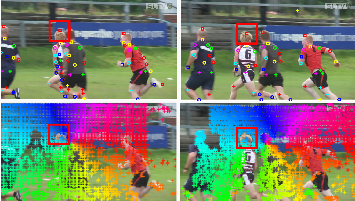
Figure 5.5: Example of the dense correspondences used for temporal potentials. The top row shows the joint detection candidates with the defined bounding boxes to extract the feature vectors for temporal association. The bottom row shows the correspondences found by the DeepMatching (Weinzaepfel et al., 2013) algorithm.
