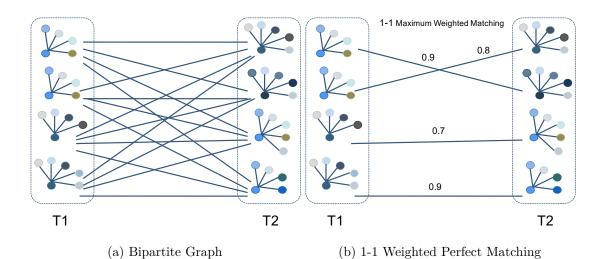
Figure 6.6: **The 1-1 Weighted Perfect Matching Problem**. The algorithm to compute the 1-1 weighted perfect matching receives as input a weighted bipartite graph where weights represent the values of a similarity measure between the RDF molecules in the bipartite graph. The output of the algorithm is a maximal matching of the RDF molecules in the bipartite graph, where each RDF molecule is matched to exactly one RDF molecule; edges in the matching have a maximal value.
