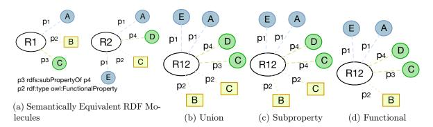
Figure 4.8: Merging Semantically Equivalent RDF Molecules. Applications of a fusion policy  $\sigma$ : (a) semantically equivalent molecules  $R_1$  and  $R_2$  with two ontology axioms; (b) simple union of all triples in  $R_1$  and  $R_2$  without tackling semantics; (c)  $p_3$  is replaced as a subproperty of  $p_4$ ; (d)  $p_2$  is a functional property and  $R_1$  belongs to the authoritative graph; therefore, literal C is discarded.
