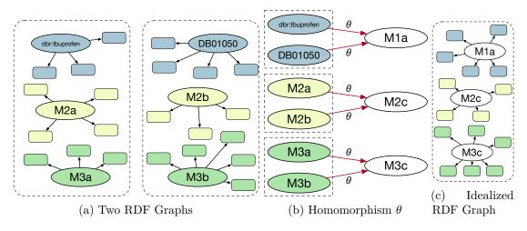
Figure 4.3: The problem of semantically integrating RDF graphs. The two RDF graphs in 4.3(a) contain semantically equivalent RDF molecules. The problem consists of building a homomorphism  $\theta$  to an idealized integrated RDF graph such as that in 4.3(c). Such a homomorphism  $\theta$  to map equivalent entities, e.g., dbr:Ibuprofen and DB01050, to an integrated entity is presented in 4.3(b).
