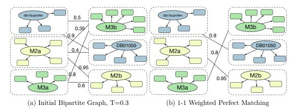
Figure 4.7: **1-1 Weighted Perfect Matching.** (a) A bipartite graph between RDF molecules from DBpedia and Drugbank; only the edges with similarity values equal or greater than 0.3 are included in the graph. (b) A 1-1 weighted perfect matching of the graph in (a); each RDF molecule is matched to the most similar one.
