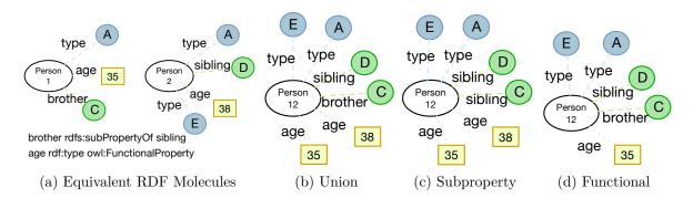
Figure 7.5: Merging Semantically Equivalent RDF Molecules. Applications of a fusion policy  $\sigma$ : (a) semantically equivalent molecules  $R_1$  and  $R_2$  with two ontology axioms; (b) simple union of all triples in  $R_1$  and  $R_2$  without tackling semantics; (c)  $p_3$  is replaced as a subproperty of  $p_4$ ; (d)  $p_2$  is a functional property and  $R_1$  belongs to the authoritative graph; therefore, literal C is discarded.
