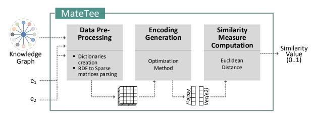
Figure 5.4: The MateTee Architecture. MateTee receives as input an RDF Knowledge Graph, and entities  $e_1$  and  $e_2$  from the knowledge graph. MateTee outputs a similarity value between  $e_1$  and  $e_2$ according to the connectivity patterns found in knowledge graph. A pre-processing step allows for the transformation of a knowledge graph into a matrix-based representation. Then, *n*-dimensional embeddings are generated. Finally, values of similarity are computed.
