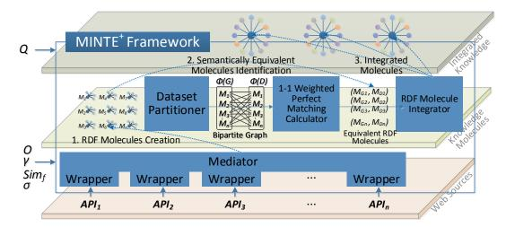
Figure 7.2: The MINTE<sup>+</sup> Implementation. MINTE<sup>+</sup> receives a set of web APIs, a keyword query Q, a similarity function  $Sim_f$ , a threshold  $\gamma$ , an ontology O, and a fusion policy  $\sigma$ . The output is a semantically integrated RDF graph.
