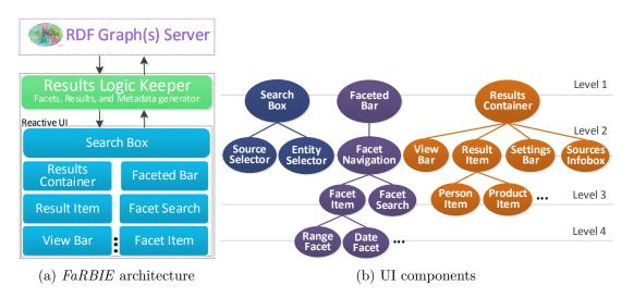
Figure 6.7: **UI Design.** (a) *FaRBIE* design contains the Results Logic Keeper and Reactive UI Components; (b) Reactive UI Components organized in levels from generic to specific. The UI components can be extended and specialized in providing a better UX according to the semantics of data.
