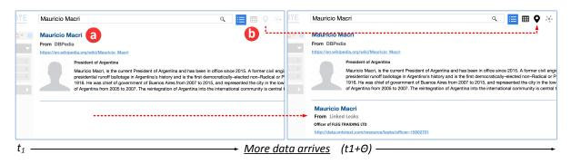
Figure 6.10: (a) **Results Container** component reacts when more data arrive. Additionally, it selects the best view according to the semantics of the results. (b) **View Bar** component reacts after analyzing the results, e.g., the map view is enabled when geo-data is found in the search results.
