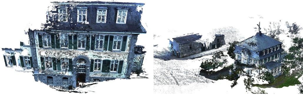
Figure 1.1: Dense 3D surface reconstruction from images acquired by an autonomously flying UAV in the project Mapping on Demand.
