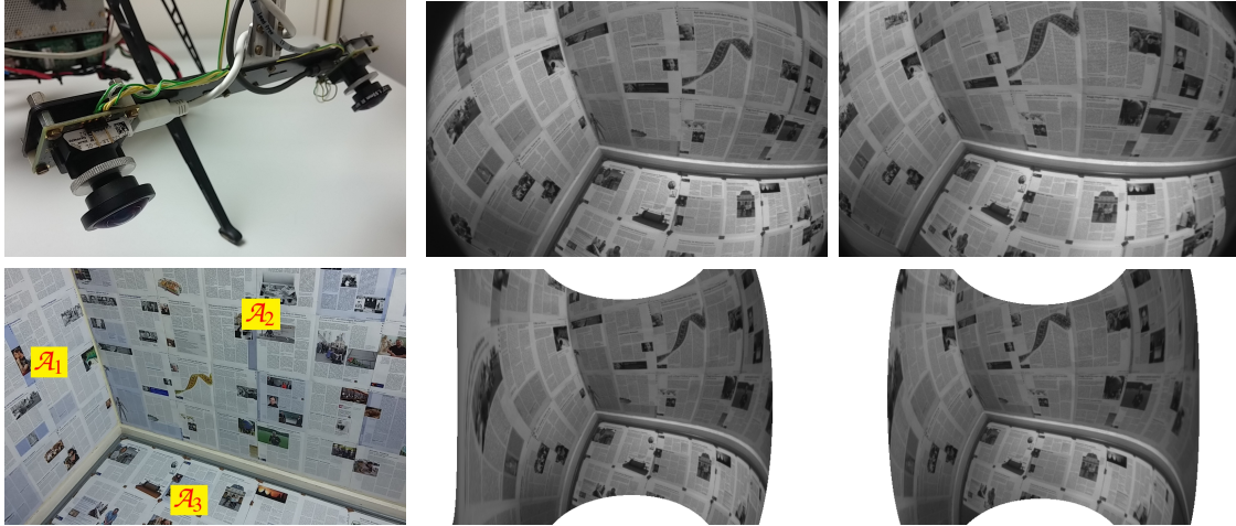
Figure 5.3: Left images: Stereo camera with fisheye lenses and highly textured and mutually orthogonal planes \mathcal{A}_1 , \mathcal{A}_2 and \mathcal{A}_3 used for variance analysis. Upper right images: Stereo image pair. Lower right: Image pair after epipolar rectification. Note that all epipolar lines of the left and right image are in the same row.
