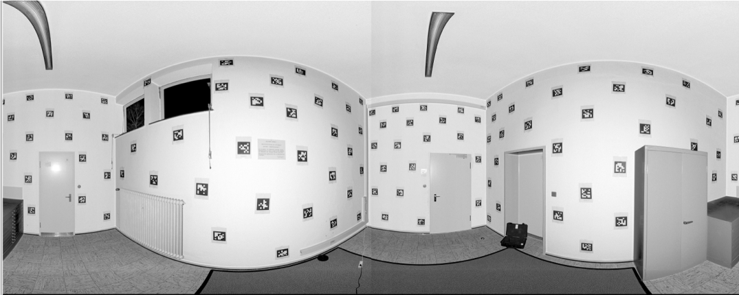
Figure 4.18: The measured intensities of a dense laser scan visualized in a panoramic grayscale image. The image allows to detect each AprilTag attached on the four walls of the room and to obtain the corresponding 3D position from the scanned point cloud.
