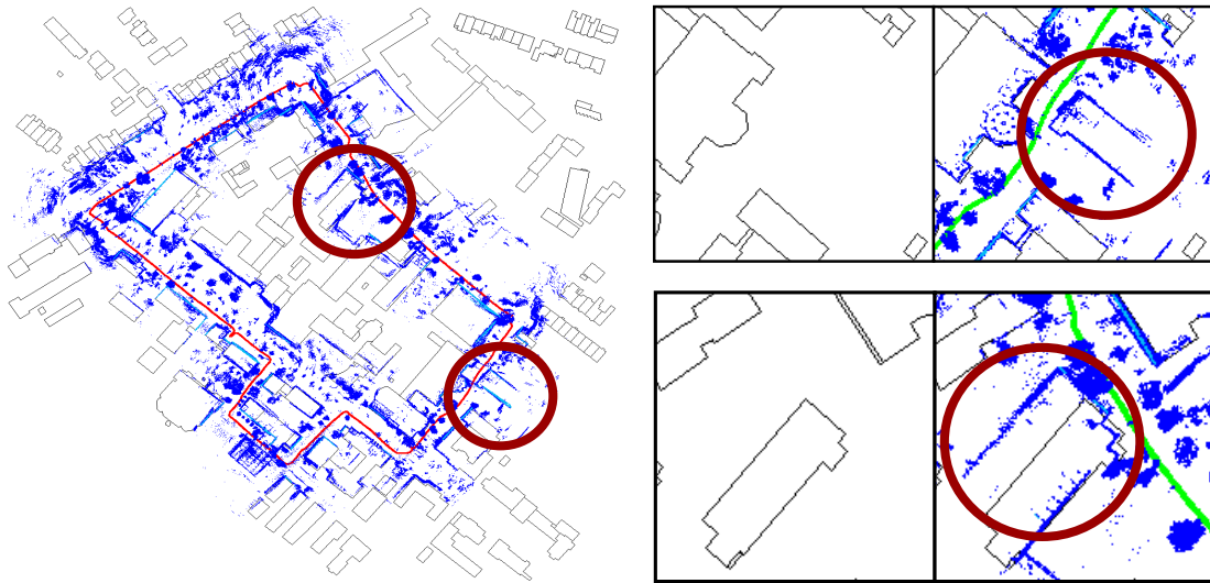
Figure 8.8: To the right zoomed views of the map inconsistencies our system can deal with. Detected buildings are marked with light blue.
