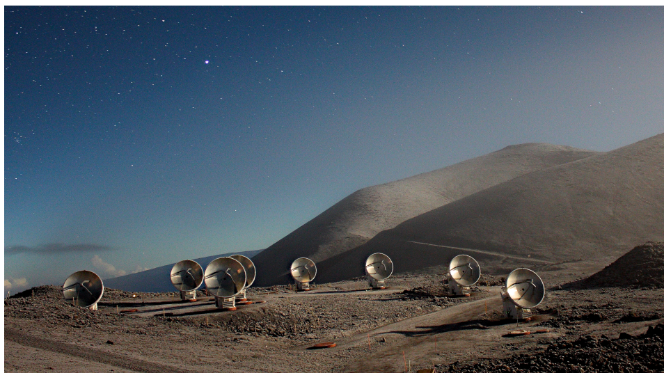
Figure 2.4: The eight 6 m antennas of the Submillimeter Array in Hawaii (USA). Photo credit: N. Patel.
