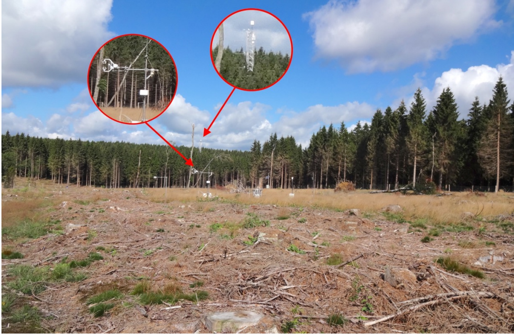
Figure 1.3.3: Photograph of the Wüstebach catchment in August 2014, one year after deforestation, facing west. The 37 m high meteorological tower with the flux measurements is situated in the spruce forest (background). A second EC station is located in the middle of the picture inside the clearcut area.
