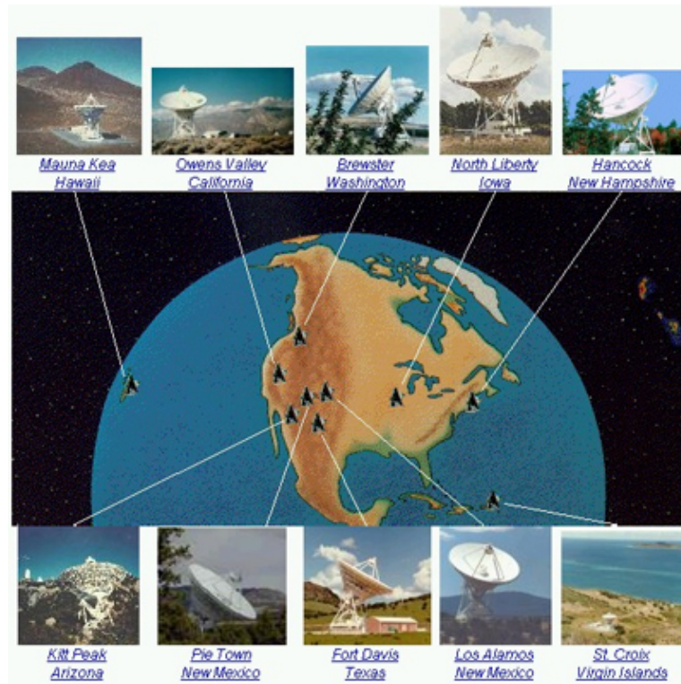
Figure 1.14: The Very Long Baseline Array consists of ten radio telescopes, each with a dish 25 meters in diameter spread over the U.S. © NRAO
