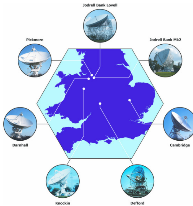
Figure 1.15: The enhanced Multi-Element Radio Linked Interferometer Network, located in the UK, is an interferometer consisting of up to 7 antennas. Image taken from http://www.merlin.ac.uk/ .
