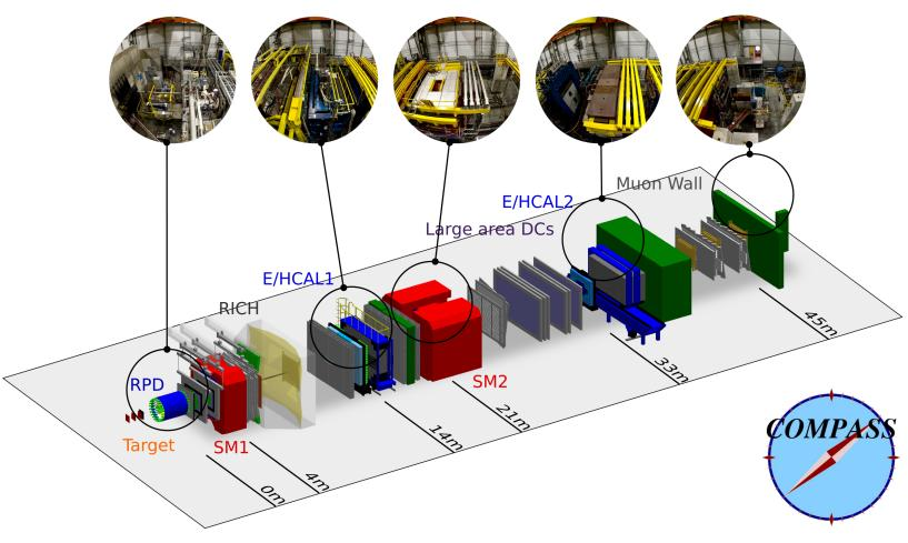
Figure 3.1: A schematic view of the COMPASS experiment setup of 2008. The 3*D*-model is exported from the GEANT4-based simulation program, TGeant described in details in Ref. [74, 75]. The panoramic photos can be found in the CERN PhotoLab, see Ref. [76].
