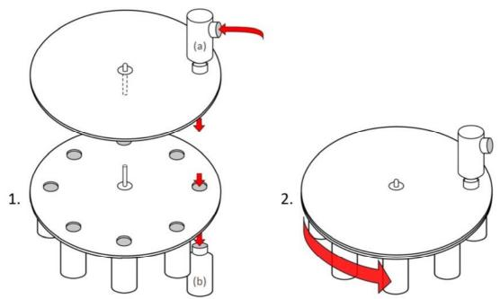
**Figure 5.2:** Concept of the revolver mechanism used in the automated interval sampler (AIS). 1. Insects are led by an adaptable trap into the capturing funnel-jar (a), from where they drop into the storing-jar (b) that is filled with high proof ethanol. 2. Storing-jars rotate in determined intervals for a temporal sample resolution.
