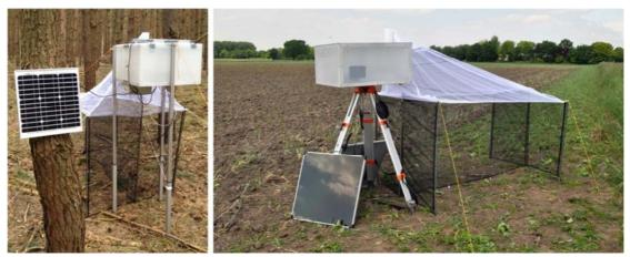
**Figure 5.13:** Left: The automated interval sampler (AIS) as it was used in the Schorfheide-Chorin together with a Malaise trap on plot SEW15 (Photo: Struwe 2015). Right: The current AIS version with improvements (Photo: Kilian 2017).
