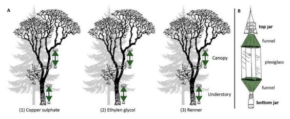
**Figure 3.1:** Graphic of the experimental setup. A: In each of the plots one tree was used for each sample solution. Two traps were installed in each tree (canopy and understory), each with two jars (bottom and top). Distance between trees within each plot was five to ten meters. Ten plots were used per tree species, beech and spruce. B: Construction of the flight interception trap used. (modified after: Gossner et al. 2014 and 2016)
