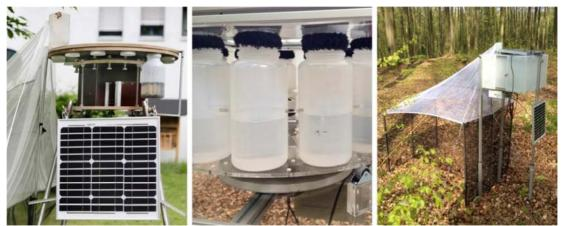
**Figure 5.1:** From left to right: (1) Prototype version of the automated interval sampler (AIS) with a single hanging storing-jar and solar panel. (2) Inside of the acryl housing of the second version with storing jars with black sealing rings fixed upon on a rotating plate filled with ethanol. (3) AIS set up with Malaise trap in the Schorfheide-Chorin on plot SEW7 (Photos: Struwe 2015).
