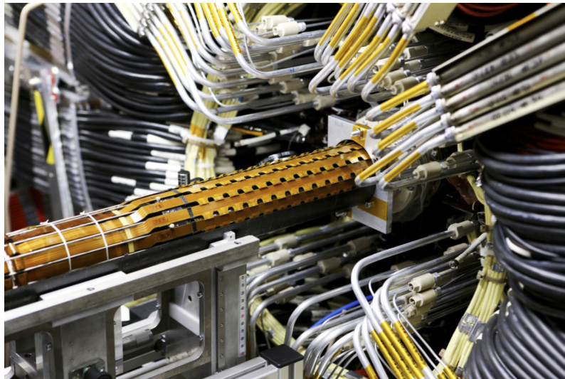
Figure 3.8: Insertion of the IBL into the ATLAS Detector in May 2014 [74].
