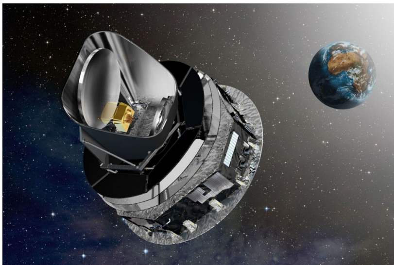
Figure 2.1: Artist's impression of the Planck satellite. Planck observed the microwave sky from the Sun-Earth Lagrange point L_2 from 2009 until 2013, completing multiple all-sky surveys. Credit: ESA
