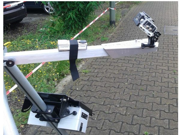
Fig. 20: Dosimeter and action camera on sensor arm (Kirchheim a.N., 21.6.2016, 10:41)
