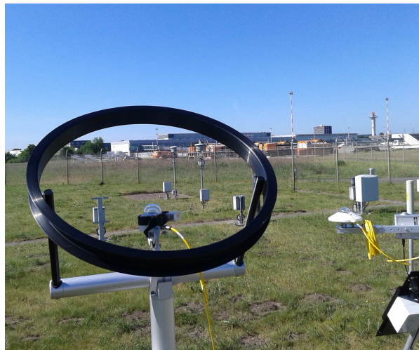
Fig. 73: Shadow ring with pyranometer and dosimeter (1.6.2017, 9:54 MESZ)
