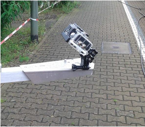
Fig. 17: Action camera attached at a sensor bar of the mobile weather station (Kirchheim a.N., 21.6.2016, 10:41 am)
