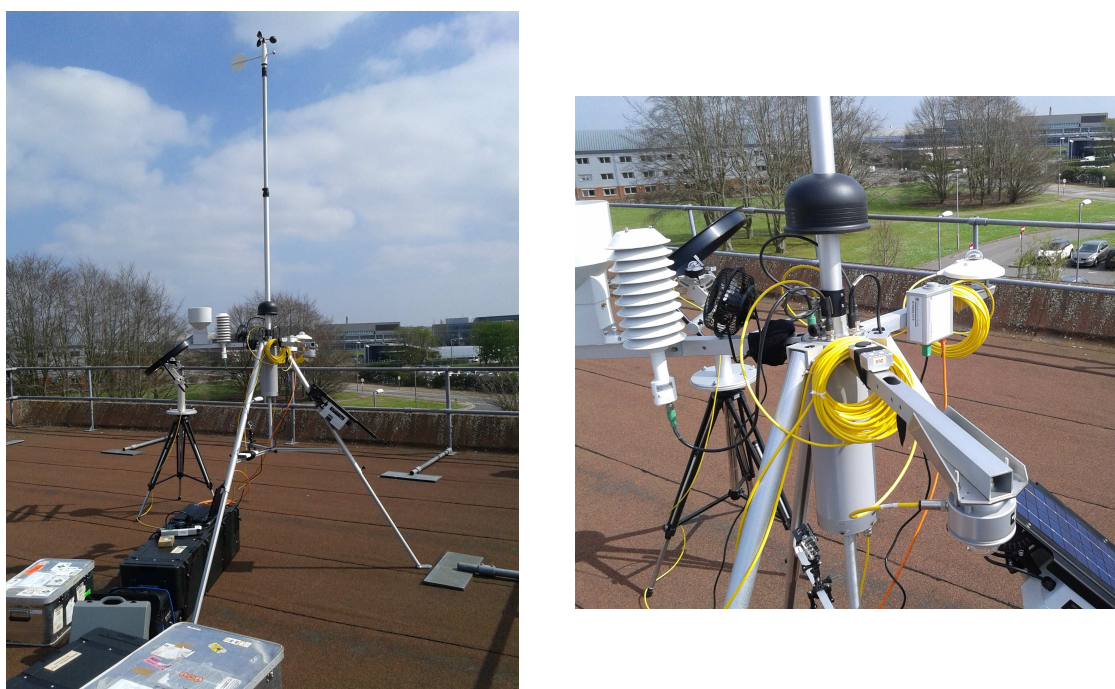
Fig. 44: The mobile weather station on 6 April 2017 on top of the PHE building in Didcot, England (left). The spectroradiometer gathering UV radiation (white box) was assembled on the sensor bar next to the pyranometer (right).
