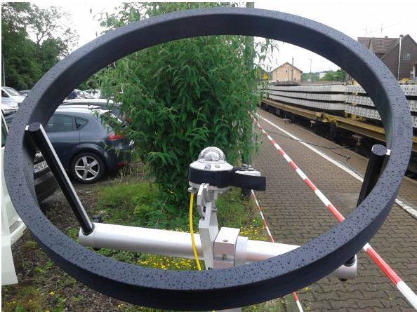
Fig. 19: Shadow ring with pyranometer and dosimeter (Kirchheim a.N., 21.6.2016, 10:40)
