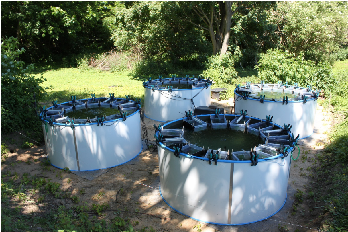
Fig. 2: Experimental set-up used for creating the two exposure treatments and animal husbandry which was used in all experiments of the present thesis. Four circular outdoor tanks (2500 l, diameter of 2 m) were arranged next to each other in a square of 36 m 2 . Within each tank, twelve enclosures were mounted serving as holding tanks for three-spined sticklebacks which were used as experimental animals. Two exposure treatments were generated by mounting a UVB lamp above every second enclosure, whereas the remaining enclosures were equipped with a dummy, providing similar shading as in enclosures with UVB lamps.
