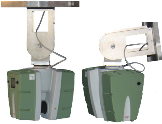
Fig. 2. Station and orientation of the TLS at an elevation angle of the telescope of 90 \text{ deg} (left) and 7.5 \text{ deg} (right).
