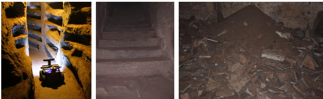
Figure 4.6: Left : robot driving in the Priscilla catacombs. Middle : non-traversable staircase. Right : non-traversable heap of rubble.
