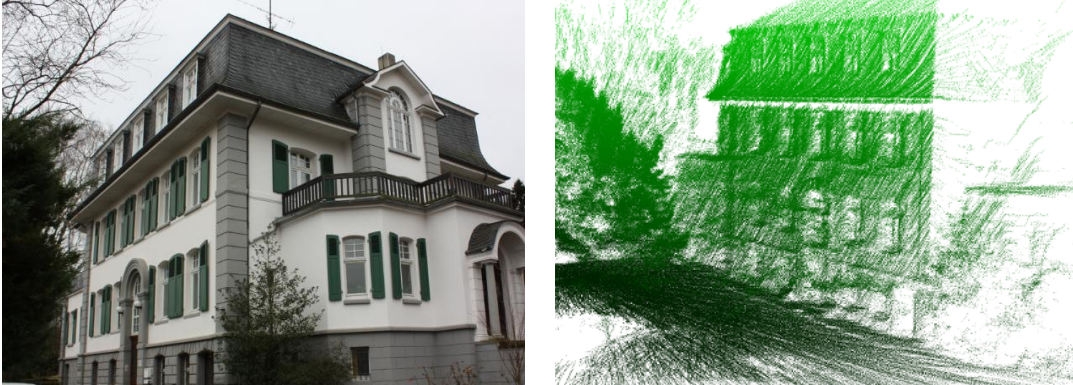
Figure 4.8.: Resulting map of the Frankenforst outdoor dataset obtained by the surfel registration (lowest MME).
