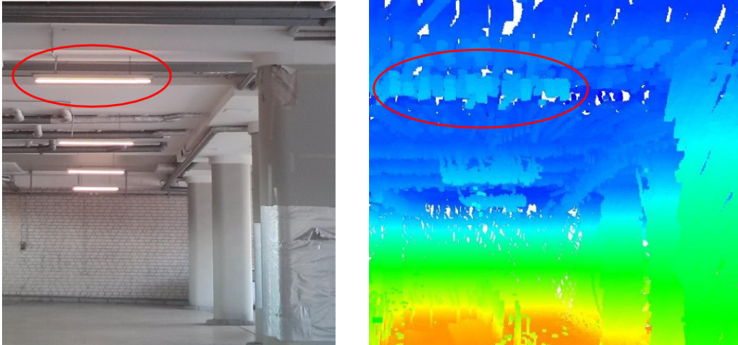
Figure 5.6.: The structure of the ceiling showing hanging lamps in a photo (left) and the resulting 3D map (right).
