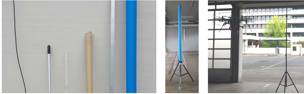
(a) Left: Different object types, from left to right: cable ( \varnothing 0.75 cm), aluminium broomstick ( \varnothing 2.7 cm), plexiglass tube ( \varnothing 5 cm), cardboard tube ( \varnothing 7.5 cm), rectangular metal rod ( \varnothing 4 cm), blue plastic tube ( \varnothing 11 cm). Middle and right: experiment setup with object holder, measuring tape and flying multicopter.
