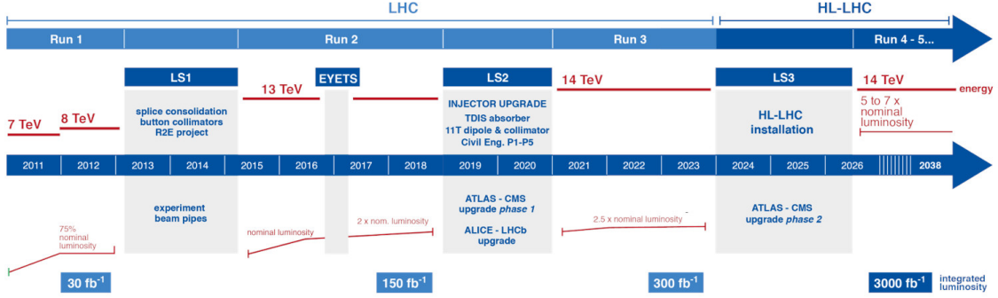
Figure 1.2: Upgrade schedule of the LHC for increased beam energy and luminosity. The total data collected for the different run periods is given by the integrated luminosity (Equation (1.5)) in inverse femto barn ( 1 \text{ fb} = 1 \times 10^{-24} \text{ cm}^2 ). Long shutdown periods of about 2 years are used to upgrade the particle detectors at the LHC.
