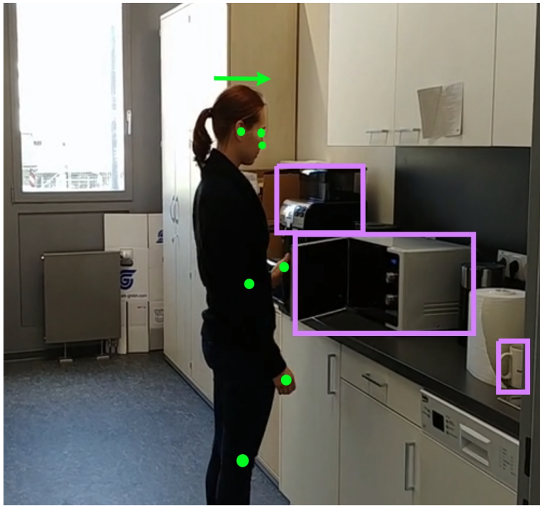
Figure 2.2: Example of the requirements to detect human-object interaction. The orientation of the human and the center of the hands is inferred based on the human pose (green). Objects (purple) that the human faces and touches (i.e., there is an overlap between the object bounding box and part of the hand positions) are marked as possible interactions. In this frame, the system will detect a possible interaction with a microwave.
