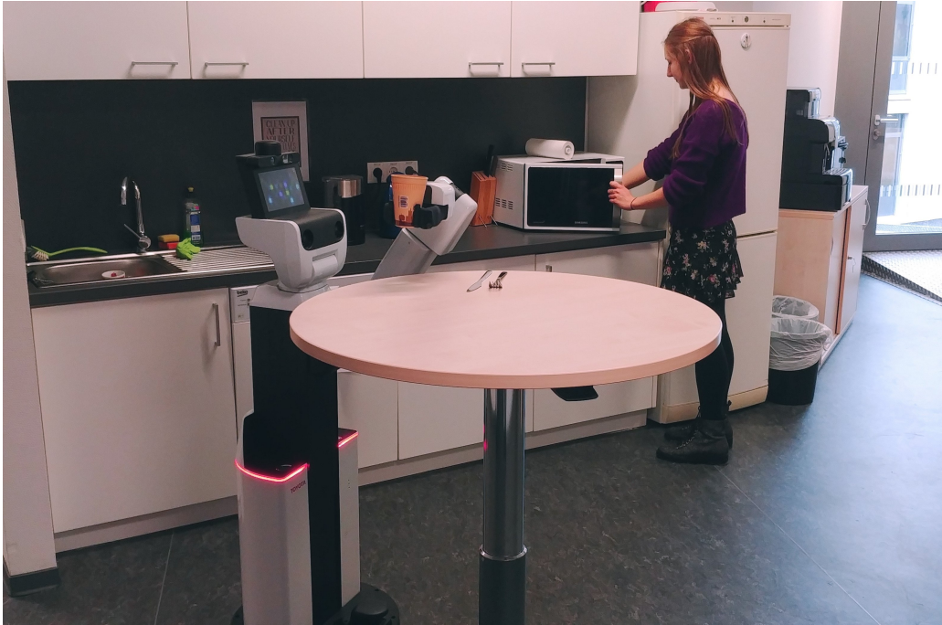
Figure 1.1: Motivational example of the presented approach. The robot observed that the user interacted with a plate and a microwave. It predicts based on observations in the past that the next object the user will interact with is the table. It also predicts that the user is likely to next interact with the table to eat on it and begins to set it, all the while avoiding positions between the user and the table to minimize the chance of interfering with them.
