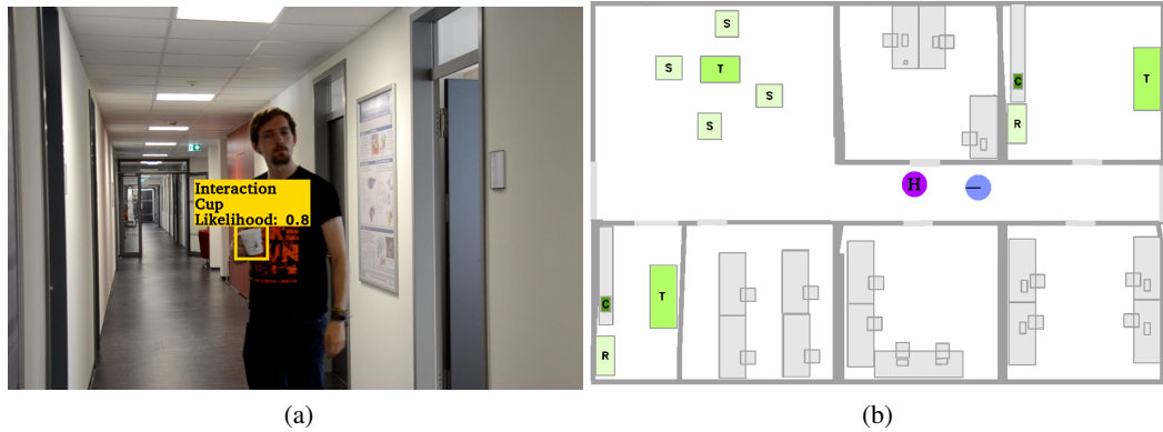
Figure 2.7: Example application of the detector to predict human movement goals. The robot (blue) detects an interaction of a human (violet) with a cup using the detection framework (a). Based on a pre-learned probability distribution about interaction transitions, the likelihood of possible next interaction objects is computed (b). The darker the green the higher the likelihood. Object names are abbreviated: table (T), sofa (S), refrigerator (R), coffee machine (C).
