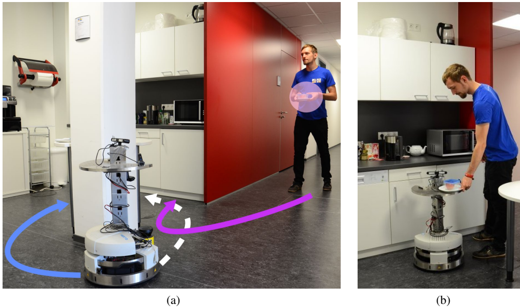
Figure 4.1: Motivating example of the approach. (a) The robot observes the moving user interacting with an object (pink circle) and predicts his most likely navigation goal and path (violet). Using the prediction, the robot is able to compute a short path to the navigation goal of the human (blue) while avoiding paths that would result in discomfort for the user (white). (b) Still, the robot arrives at the goal location before the user and early enough for direct assistance.
