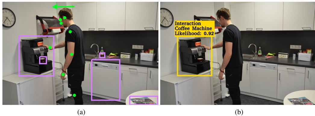
Figure 2.1: The presented detector identifies human-object interactions based on object positions (purple) as well as pose and orientation information of the human (green) (a). To deal with uncertainty in the observations, it computes for each found human-object interaction the likelihood that this interaction really occurs using previous observations (b). In this example, the human interacts with the coffee machine over several frames, resulting in a high likelihood for this interaction.
