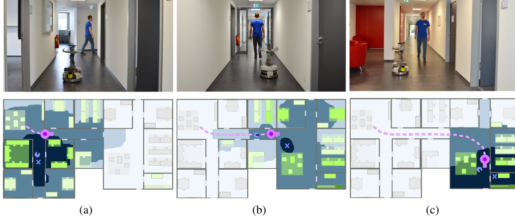
Figure 4.4: Example of the presented approach. The human (dark violet) starts their movement after interacting with a sofa. The robot (light blue) observes the interaction and starts to plan its movement with our approach. The computed likelihood of the objects to be the user’s navigation goal are shown in green, the darker the color the higher the likelihood. Cost values of possible robot positions are shown in blue, the darker the color the lower the cost. The position with the lowest cost value is shown as blue cross. (a) Based on the initial observation the robot predicts that the human will head to a nearby office and moves accordingly. However, the robot then observes that the human is moving in another direction, concluding that its initial prediction is false. (b) The robot updates the prediction accordingly and computes a new navigation goal and path to it. The robot cannot pass by the user in the corridor as it does not want to enter their SZ or IPS (light violet). As other paths are not available it chooses to follow the user at 5 meter distance. (c) Once the user reaches a wider corridor, the robot is able to pass by the user and reach a position close to their true navigation goal.
