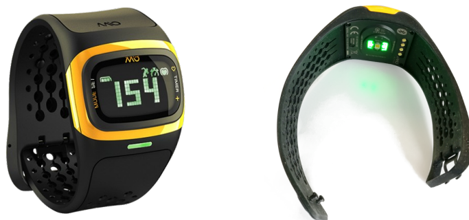
FIGURE 5.1: Mio pulse sensor [82]. The watch, compared to available watches in the market provides more accurate heart rate and in better time resolution ( 1Hz ). The watch could record for the minimum of 24h and was easy to wear. The recorded PPG based heart rate were transmitted on the fly to a phone through low energy Bluetooth.
