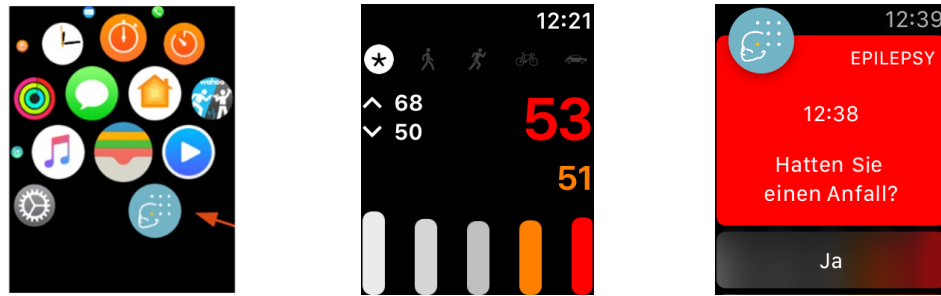
FIGURE 5.7: Apple watch epilepsy app. This app was developed to popup and ask patients about the occurrence of a seizure as soon as a suspicious heart rate change is detected. Due to very low time resolution of the signal ( 0.1Hz ), machine learning could not be applied for detecting suspicious activities. Instead, five different threshold values were used to set an alarm for different user activities. (stationary, walking, running, cycling, driving). The patient then responds to the alarm by telling whether or not a seizure took place. The patient's report could be sent to a caregivers' email by though the accompanied app from the linked iphone.
