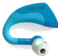
FIGURE 5.4: Cosinuss one in-ear sensor [20]. The sensor can measure PPG, accelerometry and temperature and transmit it in real-time to an external receiver. The advantage of this device was to provide raw PPG, which contained SPO_2 information (oxygen saturation). The sensor had but limitations in battery life as it had to be changed every 6 hours.
