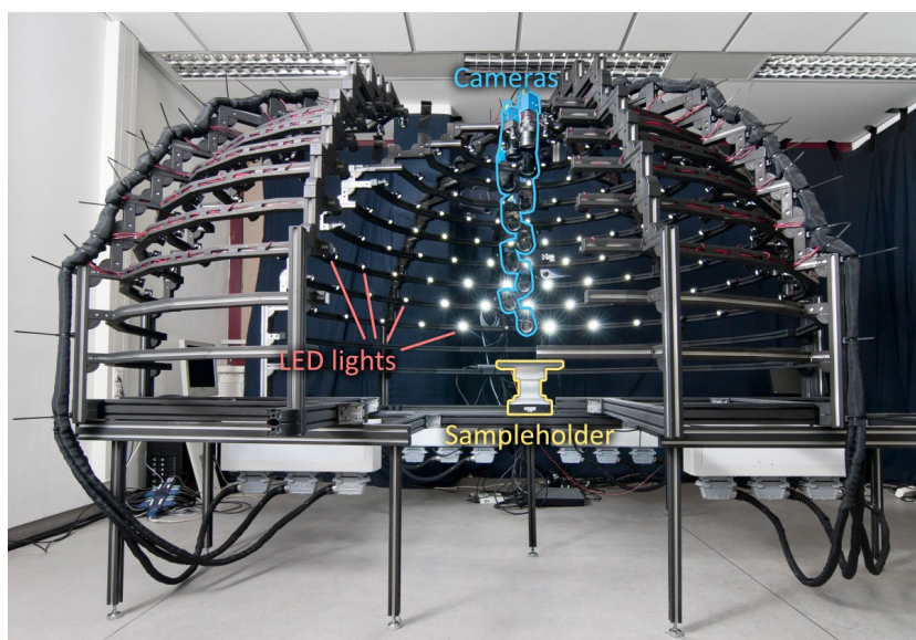
Figure 10.1: Photograph of the RGB measurement setup utilized during our experiments.
