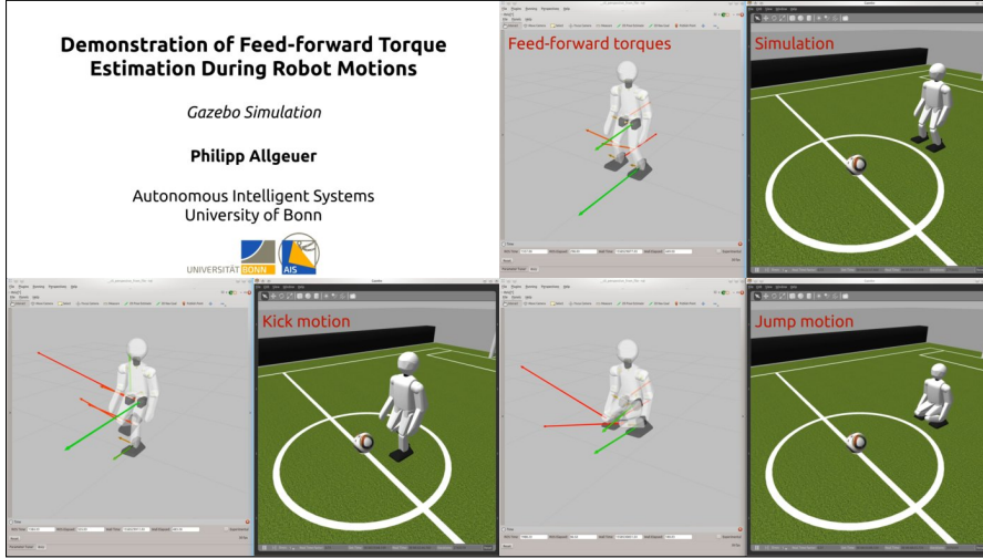
Video 3.1: Demonstration of the actuator control scheme, and in particular feed-forward torque estimation scheme, on the igus Humanoid Open Platform in Gazebo simulation.
