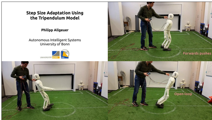
Video 11.3: Demonstration of step size adaptation using the tilt phase controller and tripendulum model. The NimbRo-OP2X is pushed repetitively in the sagittal direction and compared in performance to the same gait without step size adaptation. A plot corresponding to the second-last backwards push of the robot in the video is provided in Figure 11.7.
