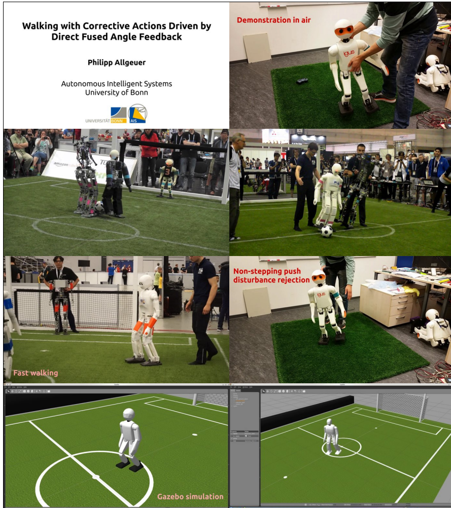
Video 9.2: Demonstration of the closed-loop direct fused angle feedback gait. Simple corrective actions based on the estimated fused angles of the torso are used to maintain the balance of the robot, even in the face of disturbances. The gait is demonstrated on the igus Humanoid Open Platform, Dynaped, NimbRo-OP2 and NimbRo-OP2X robots, as well as in simulation.
