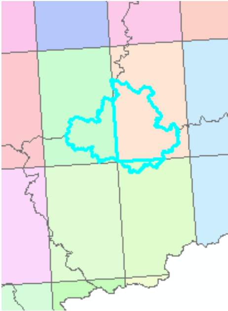
Fig. 21: Example of areal weight: The reporting area 'Dresden' is covered by three weather grid cells. The areal proportion of each grid cell to the reporting area is calculated based on the overall areal size of the latter.
